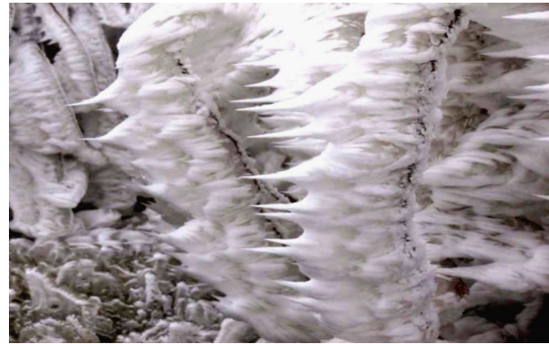
Fig. 12. Ice storm in Serbia, which caused horizontal icicles and collapsed 75 towers of 110 kV
